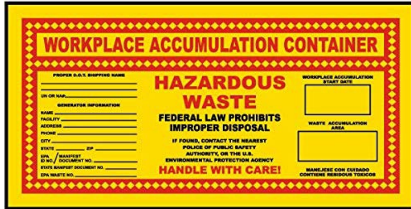
FIGURE 2.0: HAZARDOUS WASTE ACCUMULATION LABEL
