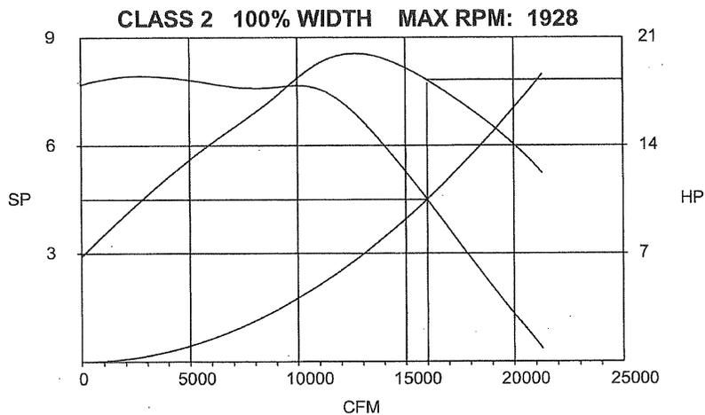
FIGURE 2 PERFORMANCE OF SMALLER FAN IN THE SAME AHU
