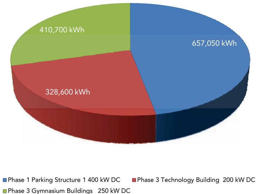
A photovoltaic system requires approximately 90 -115 ft<sup>2</sup> of footprint area per installed kW DC. In addition, this area should be free from solar shading from other buildings, trees, light poles, or other structures. Thus rooftops and parking lots are the preferred PV locations.
