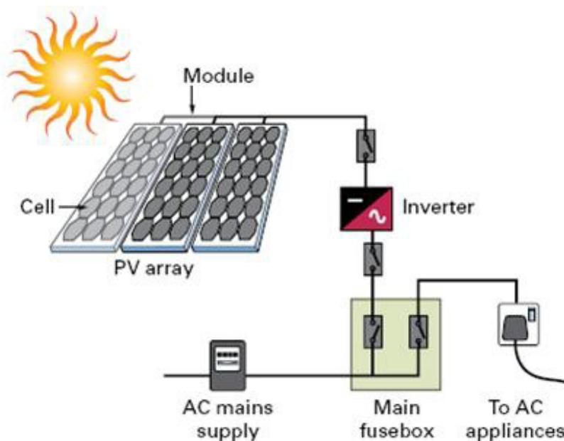
There are three main parts of a grid connected system. The biggest element is the photovoltaic panels and their support structure. The second major component is the power inverter(s). The final part is the interconnecting equipment and metering to tie the system into the power grid.
