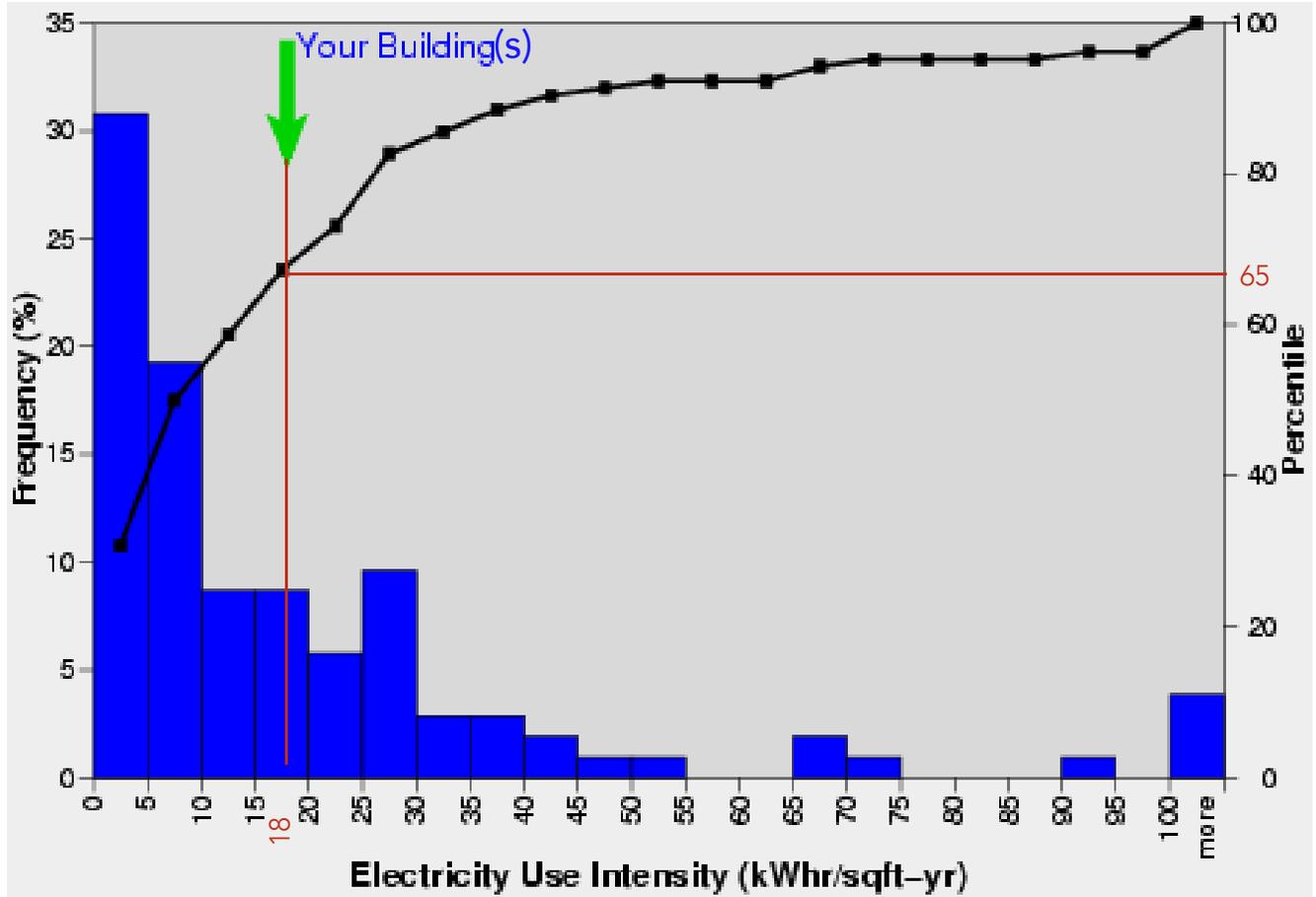
SBVC electric EUI is 18 kWh/ft<sup>2</sup>-yr is higher than 65% of comparison buildings shown in the climate zone, per database of California Building Energy Reference Tool.
